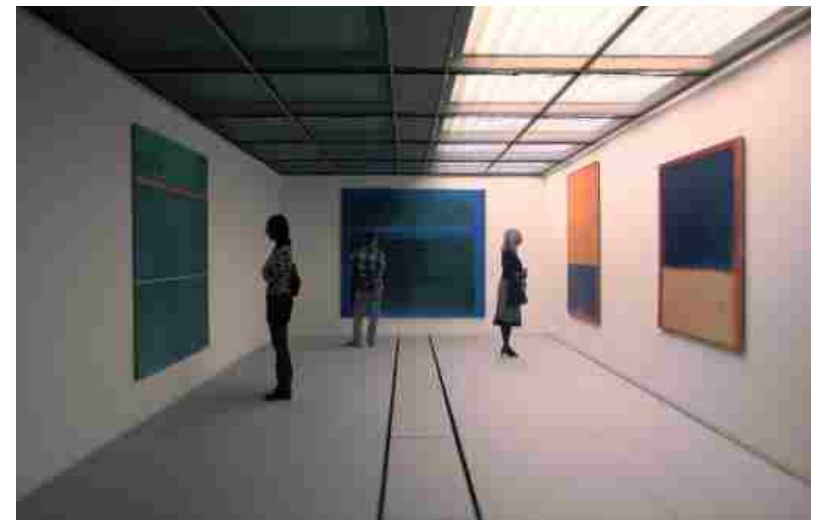
Fig: 7.16 Diffuse Sidelighting- One Side (Image of physical model taken in the overcast sky box.)
